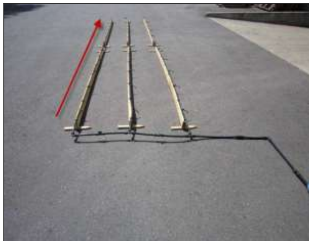
Drip Emitter Output drops down the line
