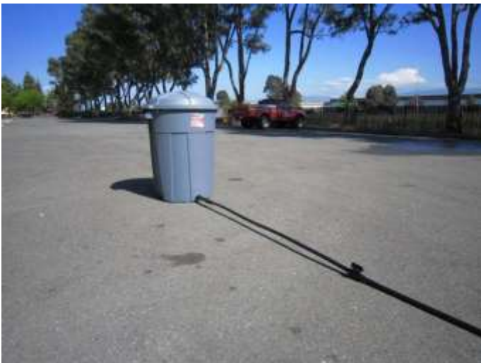
Rain Barrel with drip tubing
